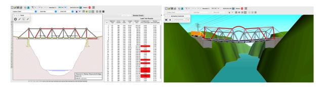
Shown above is the first prototype, and as such, is referred to as Prototype One. This bridge cost \$423,012.05. This bridge had 9 weak members (beams), primarily located along the middle parts of the top strut. There were also some diagonal beams that had stability or load issues, but those were also mainly concentrated towards the center.
