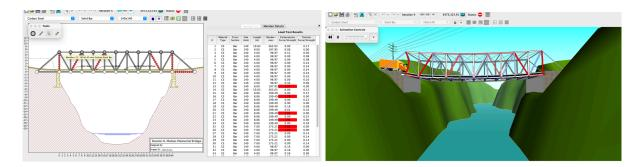
Shown above is the second prototype, and as such, is referred to as Prototype Two. This bridge cost \$473,323.91. This bridge had 6 weak members, although in this design, in opposition to the last one, they were primarily located along diagonal beams further towards the outside. In this bridge, there were more vertical beams added towards the center, which resolved the load issues with the center top strut. This version also had different spacing between the trusses.
