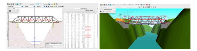
Shown above is the third prototype, and as such, is referred to as Prototype Three. This bridge cost \$550,462.54. This bridge had 5 weak members, with the largest being the beam across the center, but it still had the issue of some of the outside beams bearing too much weight. This bridge design included a center middle strut, in hopes to
